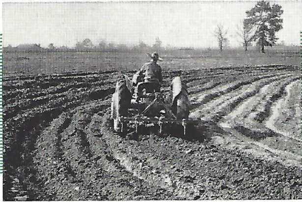
The operator of this Ford tractor with Ferguson system and All-Purpose Cultivator is a 12-year-old boy. The picture shows the unit being used to rebuild terraces.
